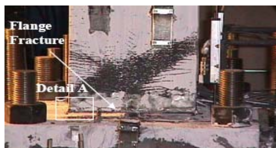
Figure 4.1 Illustration of DS-2 Brittle Fracture Propagation at Column Base Plate
