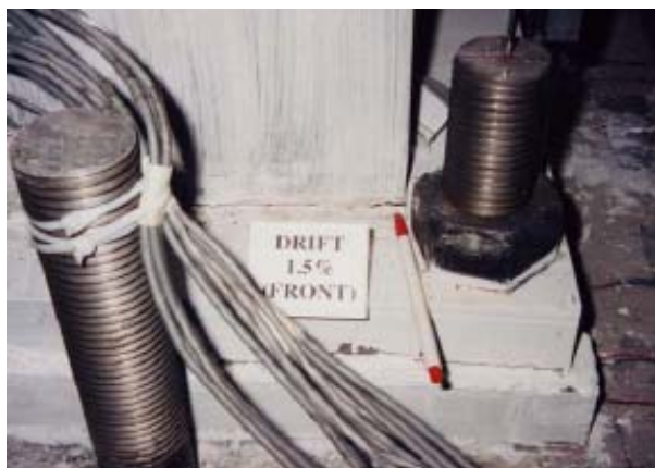
Figure 4.1 Illustration of DS-1 Fracture Initiation at Column Based Plate
